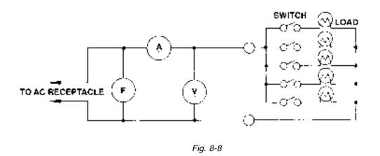
Use a circuit like the shown in Fig.8-8 for measuring AC output. A hot plate or lamp with a power factor of 1.0 may be used as a load. Adjust the load and rpm. and check that the voltage range is as specified in Table 8-2 at the rated amperage and rated rpm.
